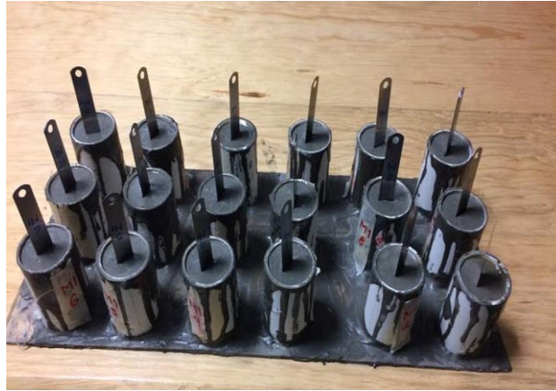
Figure 6.2 Artificial cracks in Portland cement and mortar specimens. The crack width was formed with stainless-steel shim inserted in the fresh cement paste and then extracted after the final setting of the cement paste.
