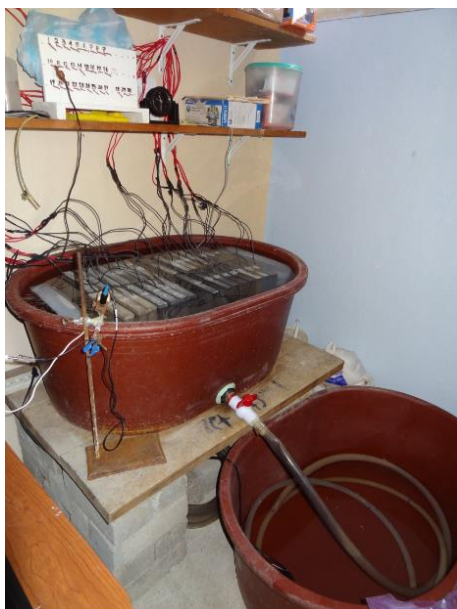
Fig. 4. The simulated marine environment for the reinforced mortar slabs
