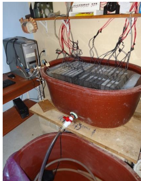
Fig. 2. Exposure conditions of the reinforced mortar slabs
