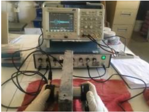
Fig. 5. The used equipment for ultrasonic measurements in the reinforced mortar slabs
