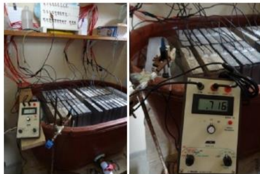
Fig. 1 Setup for the corrosion potentials measurements during the wetting cycle of the slabs.
